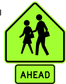
Figure 24: MUTCD S-1-1 Sign and W16-9P Sub-plate
